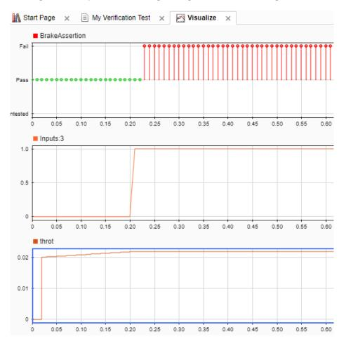
These plots show you that when the brake goes on (Input 3) the throttle stays on. The throttle should go to 0.
