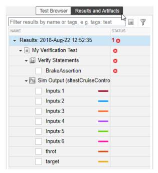
**3** Click **BrakeAssertion** and select the check box to visualize the results. You can see that the test failed at 2.3 seconds.
